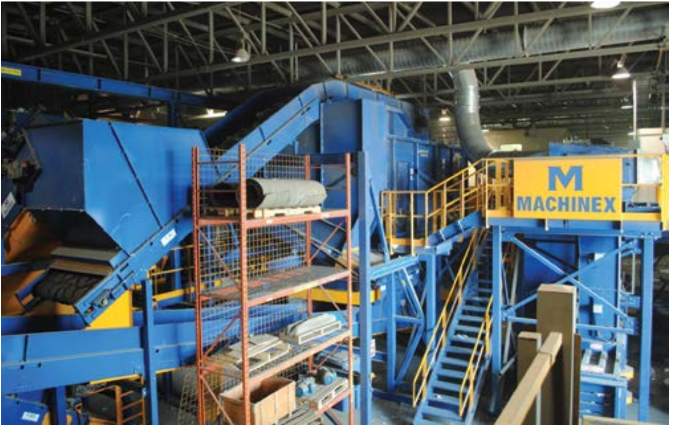
Rearview of the Mach Ballistic separator.
