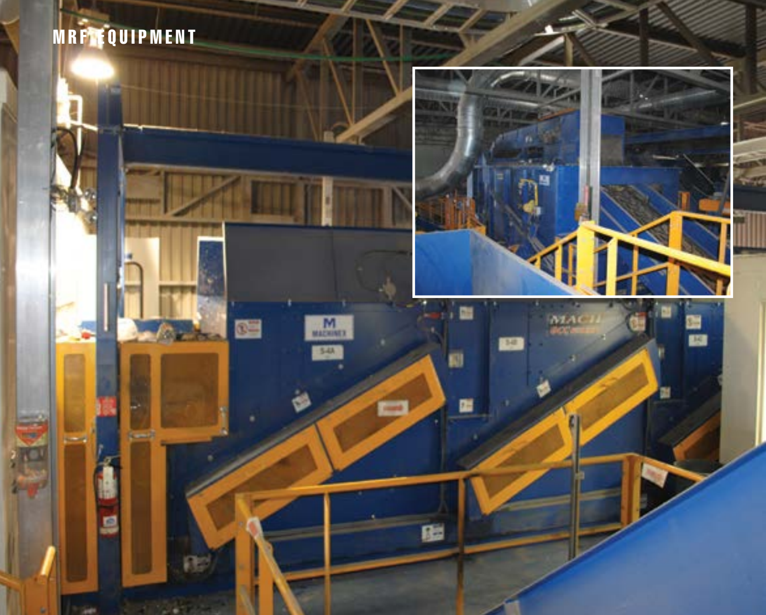
Mach OCC Disc Screen (inset: Mach Ballistic Separator).
