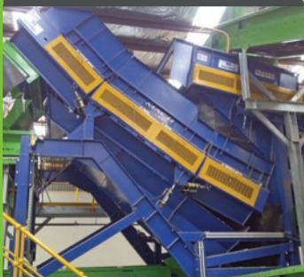
FINES SCREEN AS UPPER DECK TO A 2D FINISHING SCREEN
