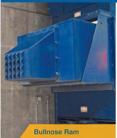
The bullnose ram prevents waste from falling on the floor and offers better compaction compared to the standard ram.
