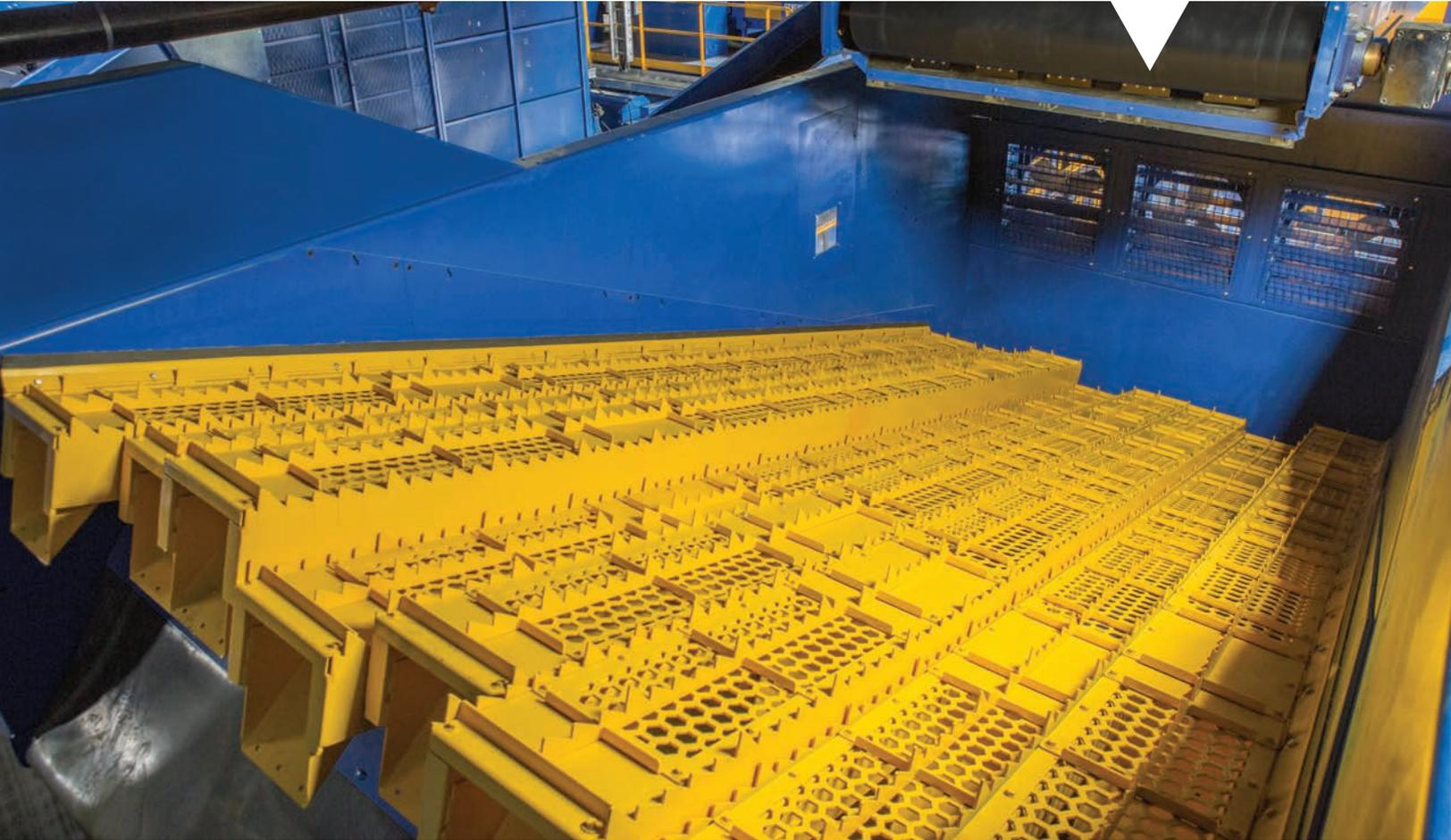
The MACH Ballistic separator is designed for sorting 2D material (plastic film, paper, cardboard, and fibers) from 3D material (containers, plastic bottles, cans, stone, wood, etc.). While the 2D material travels up this slope with the paddles, the 3D material bounces or rolls downward. Fine particles can be collected separately with the optional variable screen openings.
