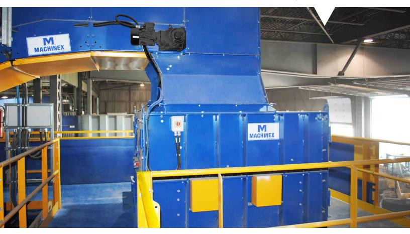
The Machinex bag opener is an essential equipment when comes the time to process material that is totally or partially bagged. Located at the front end of the system, it can be integrated in-line when all material is bagged, or as a backup unit on which only bagged material is diverted. Its two rotating blade shears the plastic bags, liberating material without damaging the recyclables.
