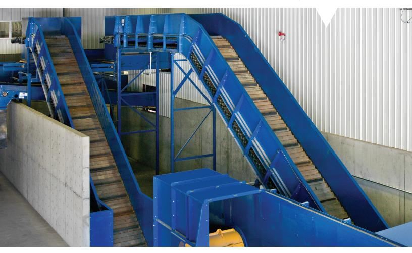
The chain roller conveyor is typically used for infeed, as well as baler feeding.
