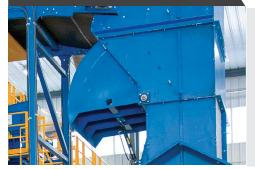
The jam breaker helps keep material moving freely through the feeding hopper. The device uses infrared photocells to ensure automatic clearance of the feeding hopper and eliminate fastidious release operations.
