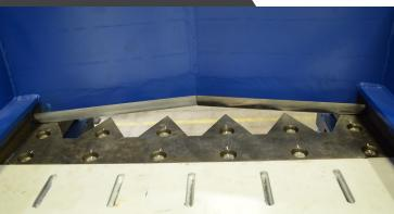
The two pieces fixed knife form a "V" which helps to cut material progressively. The mobile knife is made of one piece including 5 pointed teeth with an underneath clearance angle.
