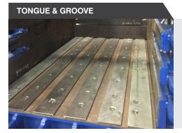
The stepped profile of the tongue & groove floor greatly reduces the possibility of thin material lid to penetrate under the ram. This helps to keep the gap between the knife very tight and at the same time reduces the maintenance cost.
