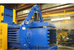
The optional heavy duty extrusion chamber includes a 230 tons cylinder.
