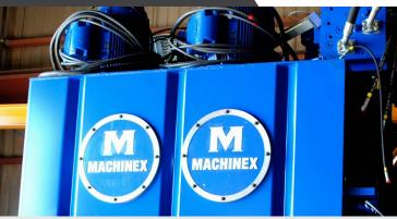
The totally enclosed, fan-cooled (TEFC) motors work efficiently in dusty conditions and poor ventilation.
