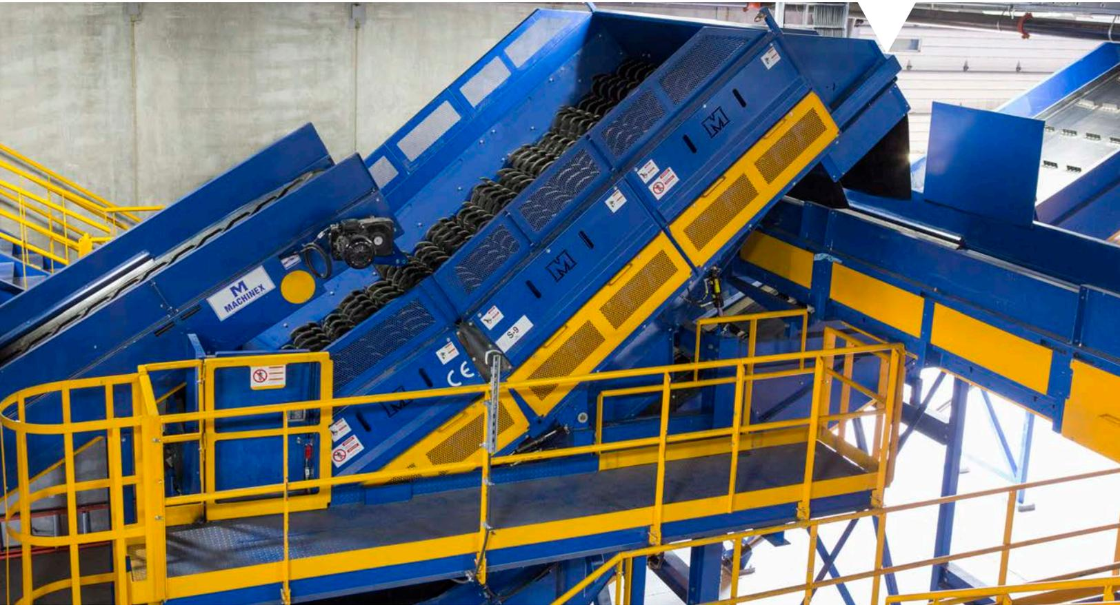
MACH One News disc screens separate fibers and containers while removing a maximum amount of newsprint from the material stream. They can also be used on other types of systems, such as municipal solid waste, fiber sorting facilities and other streams that contain fibers.
