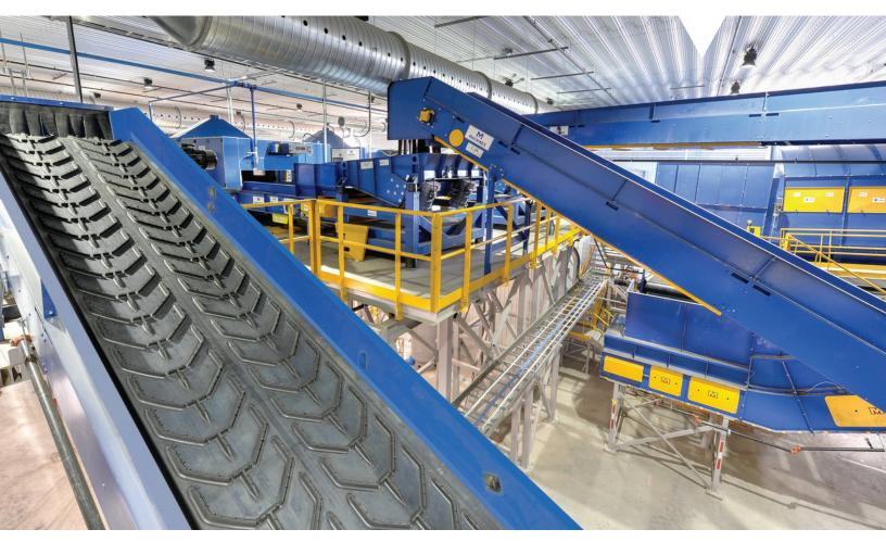
The picking idler conveyor is the perfect piece of equipment for carrying fine and abrasive particles, such as glass and other aggregate. Its inclined sides allow for a high holding capacity and belt types are specifically chosen to fit your needs.
